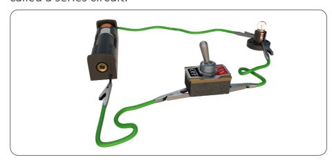
When electricity flows through all the components of a circuit, it is called a complete circuit.
